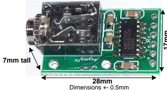
A very small TTL to RS232 adapter with a 3.5mm jack. Available as a TTL 5v IC232 or TTL 3.3v IC3232
