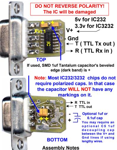
Use quality solder approx .020" dia and a fine point soldering iron approx 20w.
