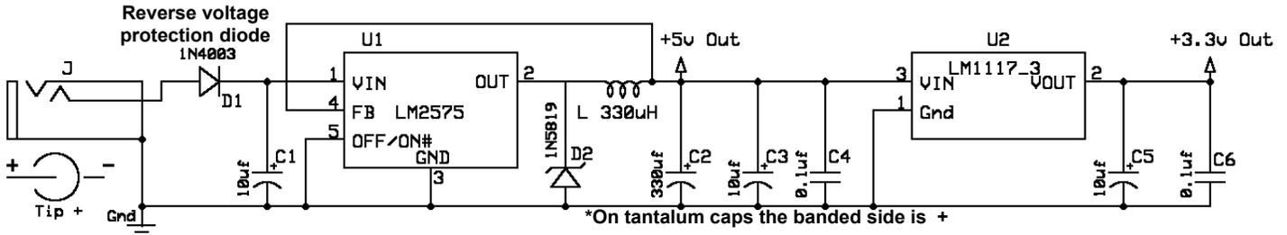
Note: Power LED not shown in the schematic. Banded end (green stripe) is the cathode
