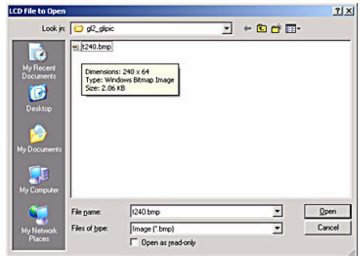
**NOTE:** If you draw images/text in the graphic area you *MUST save the file as a bmp image and then re-load it before it can be sent to the LCD.* If you plan on using other images make sure that they are 1 bit color (B/W) with a resolution of 240x64 bits which is the resolution for the supplied demo code.
