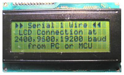
Use with 1,2,3 or 4 line displays. (Four line LCD shown above)
