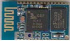
The BTM-182 module is a versatile and inexpensive bluetooth device. It is a Class 2 module with printed pcb antenna, *Bluetooth* standard Ver. 2.0 + EDR compliant. Low current consumption, 3.0V or 1.8V operation. Possible Interfaces: USB, UART & PCM (for voice CODEC), RoHS compliant. Small outline. 25.0x14.5x2.2 mm
